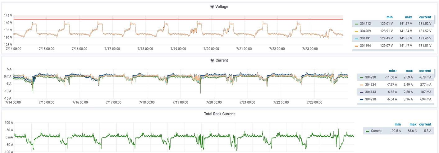
Image / Sample Screenshot displaying types of information accessible through Powerlink
